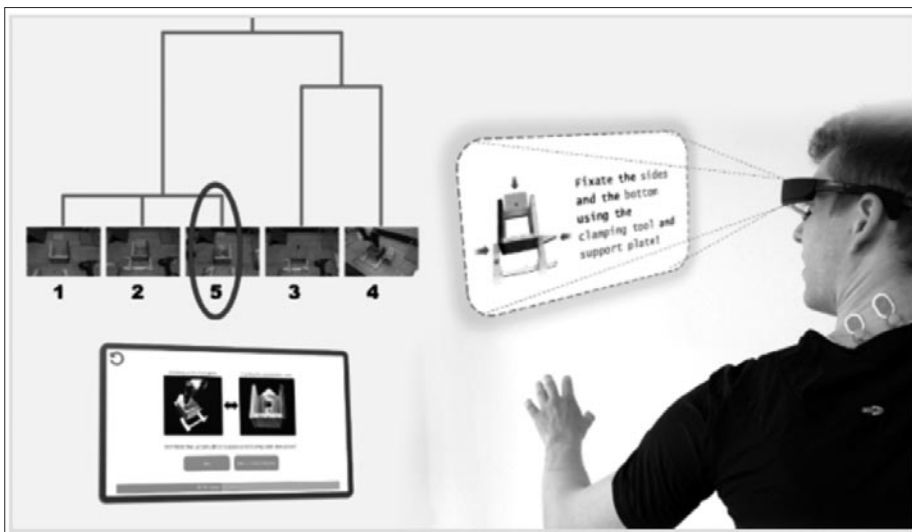
Fig. 2. - The basic idea behind the cognitive ADAMAAS-Glasses: Mental representations are evaluated in advance with the help of the SDA-M diagnostic on a tablet PC (left). A particular computational algorithm is then estimating the probability of failures in different steps of a particular action (e.g., building a nesting box). Relevant and individualized prompts are provided in time in the AR component of the glasses to support anticipative processing of the user (right). Photo: CITEC. Reproduced with permission of Thomas Schack.
